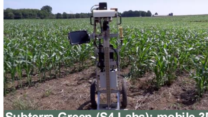
Subterra Green (S4 Labs): mobile 3D soil carbon mapping to 90 cm using VNIR and force sensing.
